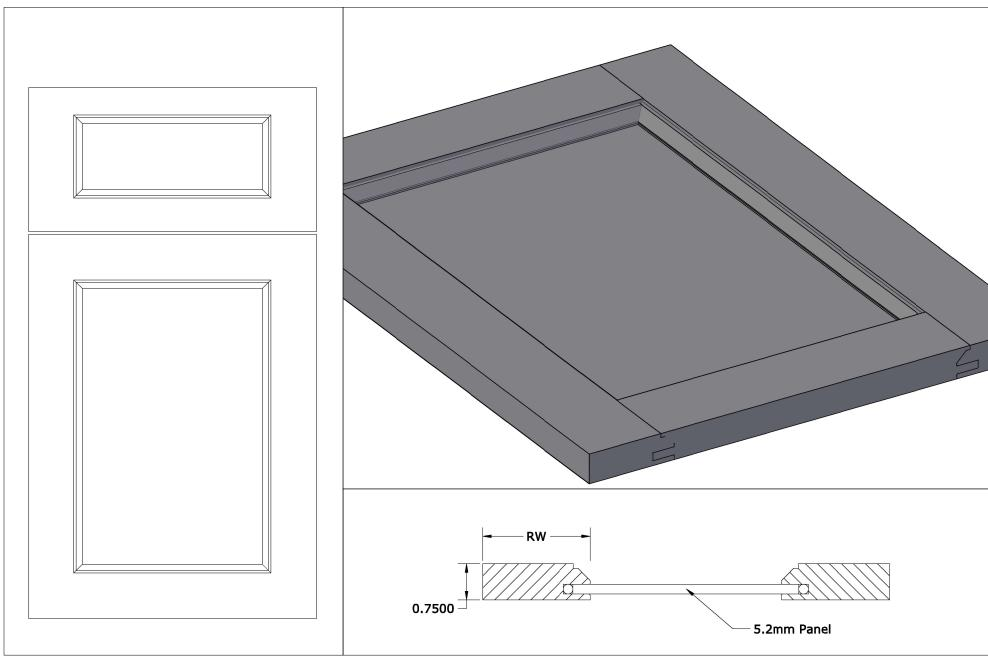
\*Standard 3/4" finished thickness \*Drawer front panels have horizontal grain \*Drawer fronts <7" tall have standard 1-1/2" top and bottom rail
